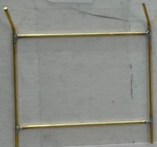
0.81 mm (1/32") brass wire Cut and soldered
